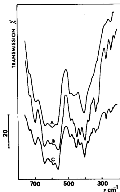
FIG. 3. Comparison of infrared spectra of defect spinels with the same number of vacancies ( x = 0.16 ). A: (\text{Fe}^{3+})_A(\text{Co}_{0.16}^{2+}\text{Fe}_{1.36}^{2+}\square_{0.26})_B\text{O}_4^{2-} . B: (\text{Zn}_{0.16}^{2+}\text{Fe}_{0.84}^{3+})_A(\text{Fe}_{1.72}^{3+}\square_{0.28})_B\text{O}_4^{2-} . C: (\text{Fe}^{3+})_A(\text{Fe}_{1.36}^{3+}\text{Fe}_{0.16}^{2+}\square_{0.28})_B\text{O}_4^{2-} .
